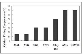
A commonly used test is that in ASTM G48, which measures resistance to a solution of 6% ferric chloride, at a temperature appropriate for the alloy, shown in the graph above. If an artificial crevice is added to the sample the test measures crevice corrosion resistance rather than pitting resistance. The temperature which is just high enough to cause failure of this test is termed the Critical Pitting Temperature (CPT) or the Critical Crevice Temperature (CCT).
